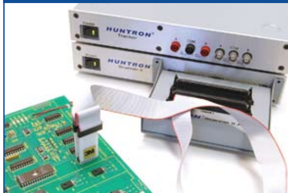
Huntron Tracker Model 30 shown with Scanner II (Scanner Adapter mounted to the front allows for connection of IDC-style cables)
